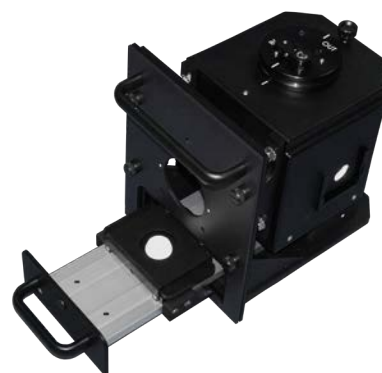
QuantaPhi-2 shown with bottom loading sample tray for powders and solids
