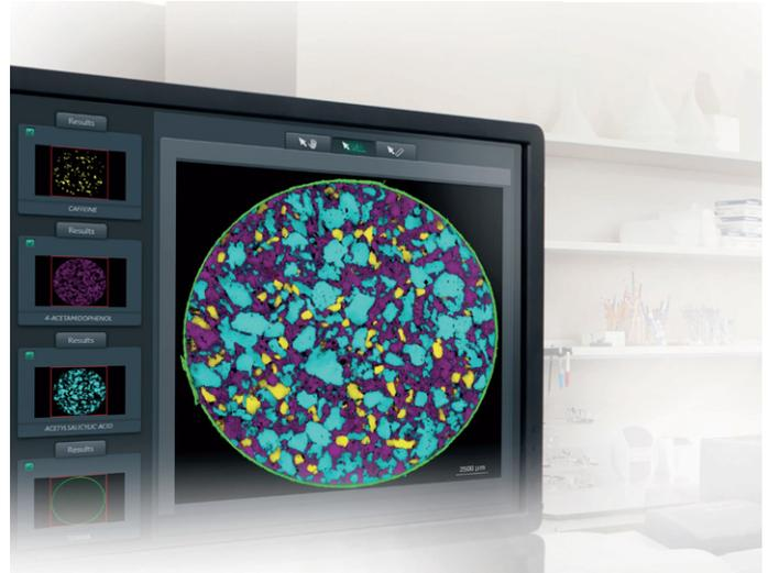
High-spatial resolution image of pain-relief medication visually pinpoints the location and quantity of four principal components with built-in Multivariate Curve Resolution. 5.4 million spectra collected at a rate of 540 spectra per second over an 11 × 11 mm area.
