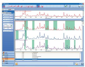
In a single step, OMNIC Specta determines the identify of the three active ingredient in a mulicomponent table: acetaminophen, acetylsalicylic acid, and caffeine.
