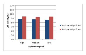
Figure 4. Aspiration speed vs. cell viability with adherent cells
