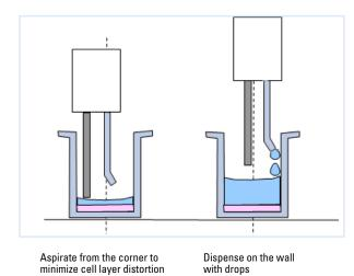
Figure 1. Aspiration mode, height, speed and time, and dispensing height and well position are adjustable in Wellwash Versa cell wash protocols.
