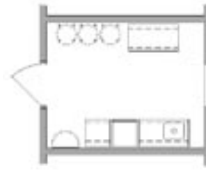
▲ Floor plan for an ideal disinfection room. Scale 1:100
