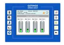
Getinge Online for remotely checking system parameters and monitoring, e.g. notifications which sends an email and/or text (SMS) message to the customer's mobile phone or PC when Getinge CMS reaches ordering level or gives a warning alarm before levels reach a critical point.
